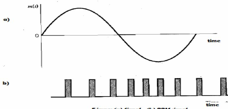
Figure: (a) Signal (b) PPM signal
